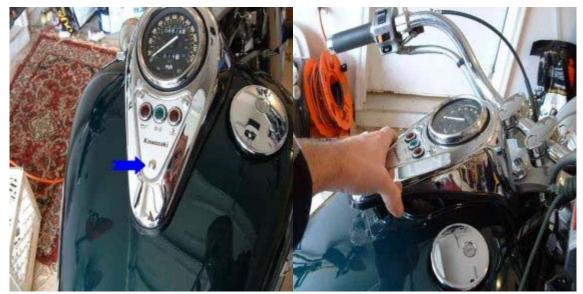
**a.** Remove the 8mm bolt at the bottom of the instrument panel (the triangular panel that holds the 3 indicator lights) on the speedometer pod. Carefully lift the rear of the pod and push forward to release the clip holding the pod at the front of the tank. Tilt the pod to allow access underneath.
