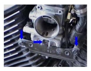
**b.** Remove the 2 10mm bolts holding the airbox mounting bracket/carburetor stop in place. *Caution*: These bolts are harder than the cylinders they are threaded into; be *very* careful not to strip the threads inside the cylinder. Set bolts aside someplace safe. Note the position of the rubber tab holding this bracket into place against the carburetor. Carefully remove bracket from carburetor and motor. Set bracket aside someplace safe.
