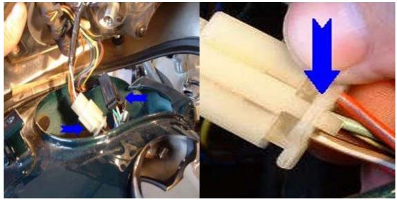
**2.** Unhook the 2 wiring harness connectors. Each connector is locked together by a slot-tab arrangement at the junction; push down on the tab and carefully pull backwards on the other half of the connector. *Do not pull on the wiring*. Lift the pod clear of the tank and put it aside someplace safe.
