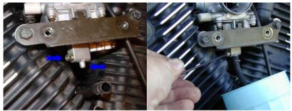
**a.** Drain fuel from carburetor float bowl by opening the 3mm Allen head bolt (carburetor drain plug) next to the small nipple on the bottom of the carburetor (carburetor drain). Catch this fuel in a non-flammable container (do *not* use a Styrofoam cup; gasoline will dissolve Styrofoam). Dispose of this fuel safely and immediately. Tighten drain plug.
