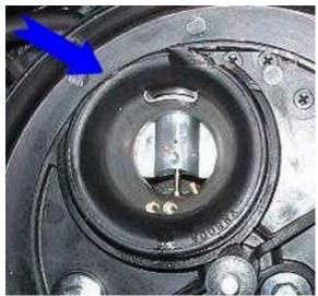
Note the position of the black rubber boot between the backing plate and the carb, and that the boot *is* rubber and *must not* be damaged. Set the backing plate aside someplace safe.
