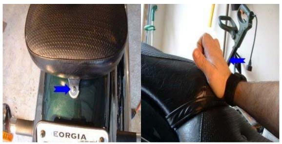
Remove the 8mm bolt at the rear that holds the back of the seat onto the fender. Strike the back of the rider's section of the seat (the "step" where it comes up to become the passenger seat) solidly toward the rear of the bike to release the clips holding the seat onto the U-bracket on the rear fender. Lift the rear of the seat and pull backwards; the front tab will come out from underneath the rear bolt of the fuel tank. Set the seat aside someplace safe.
