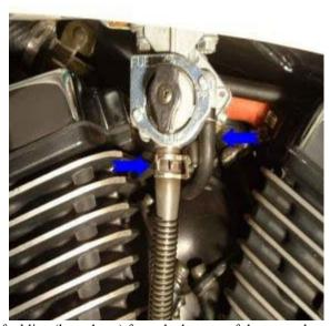
**b.** Disconnect the main fuel line (large hose) from the bottom of the petcock on the left side of the tank.
