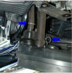
**b.** Disconnect and label the crankcase vent line (small hose) and the air switch valve line (large hose) from the rear of the backing plate.
