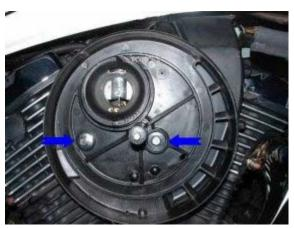
**d.** Remove the 2 10mm bolts holding the backing plate to the securing bracket in front of the carburetor. Set these bolts aside someplace safe. Carefully ease the backing plate off the carburetor.
