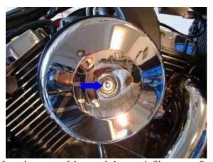
**a.** Remove the 10mm nut and washer from the center of the round chrome air filter cover. Set nut and washer aside someplace safe. Remove the air filter cover and set it aside someplace safe. Remove the OEM air filter.
