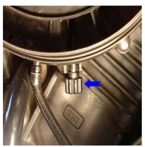
c. The idle RPM adjust is a black plastic knob hanging to the lower right of the backing plate; it is secured on a small clip to the rear of the backing plate. Pull the line clear of the clip and allow it to hang. Disconnect the crankcase vent line from the bottom of the airbox (this is the line that leads to the "milk bottle" at the right front of the frame).
