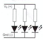
Parallel connection with each LED running from the power supply. Calculate **R** for each LED separately as above (but usually the same).
