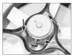
5.8 Fan motor-to-shroud nuts (arrowed)
