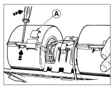
11.8 Heater blower unit locking clip (A) removal
