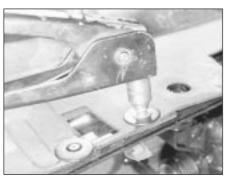
7.12 Pop-riveting the anti-splash shield to the radiator
