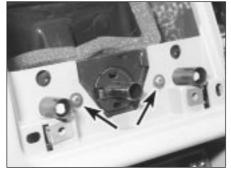
12.3A Control panel retaining screws (arrowed)
