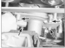
10.5 Unscrew the bolts (arrowed) to remove the water pump
