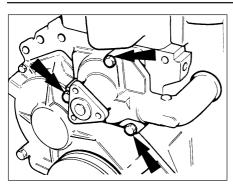
8.6 Unscrew the water pump retaining bolts (arrowed)
