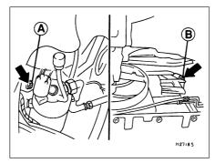
14.58 Left-hand (A) and right-hand (B) fan motor-to-support frame retaining nuts (arrowed)
