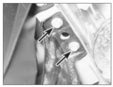
7.8 Radiator retaining bolts (arrowed)
