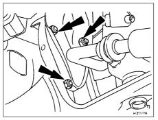
7.7B Air conditioner condenser retaining nuts (arrowed)
