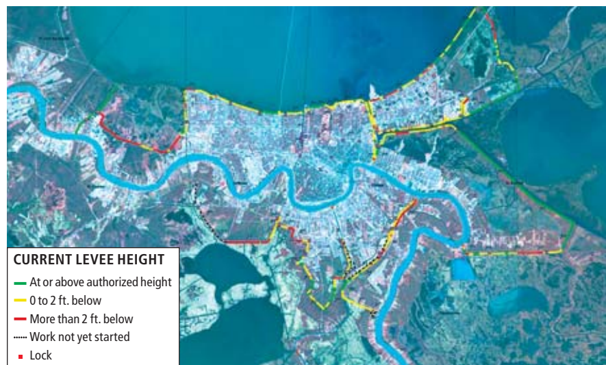
LEVEES in New Orleans have been repaired, but the entire system is subsiding below its original design height, which only offered protection against a Category 3 hurricane.
