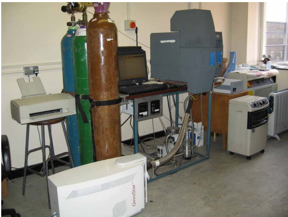
Figure 3.3 Combined facility of TG/DSC/MS
