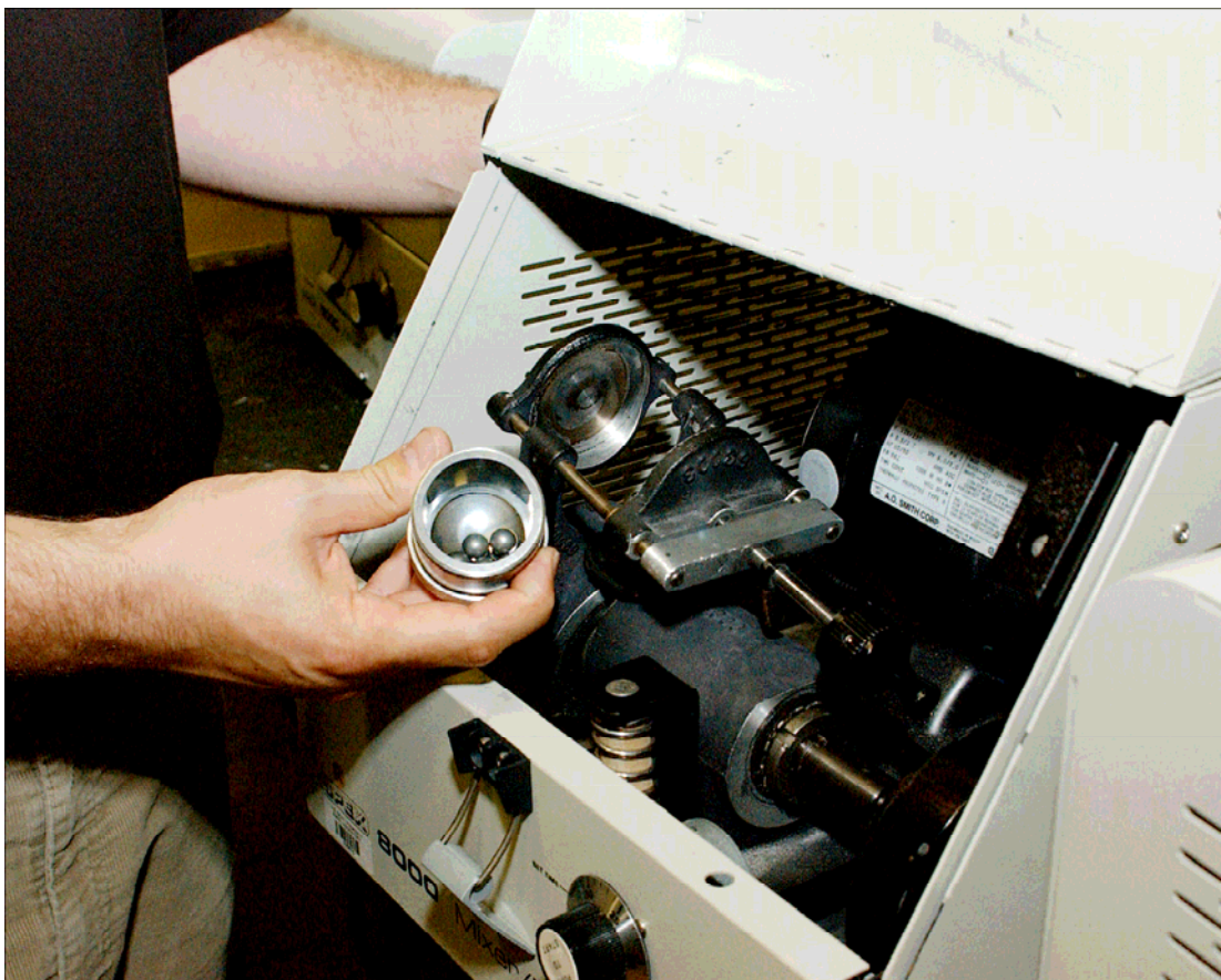
Figure 3.1 Spex-8000 ball mill Low-tech chemistry with a high payoff High-energy ball-milling, a relatively low-tech process in which metal balls are sealed in a vial with chemicals and shaken to produce new substances, may replace solvents in certain chemical reactions, offering at least a partial alternative to the use of toxic compounds such as benzene. [Environmental Health Perspectives, V. 111 (10) August 2003, pg. A534]
