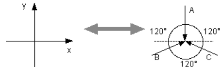
Fig. 8. Relation between [x, y] and [A, B, C] bases.
