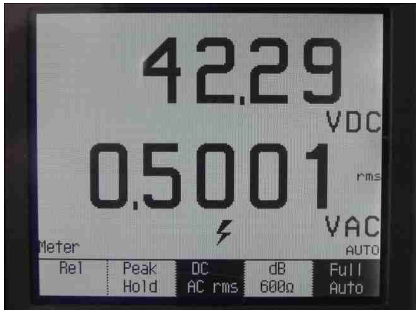
Fig028. The supply voltage drop and ripple increases.
