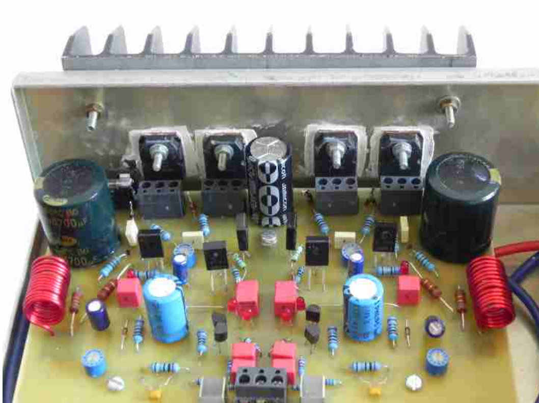
Fig005. The power transistors are fixed with insulation and thermal paste to the front face on which is attached, on the outside, the radiator. Not very elegant but enough here.
