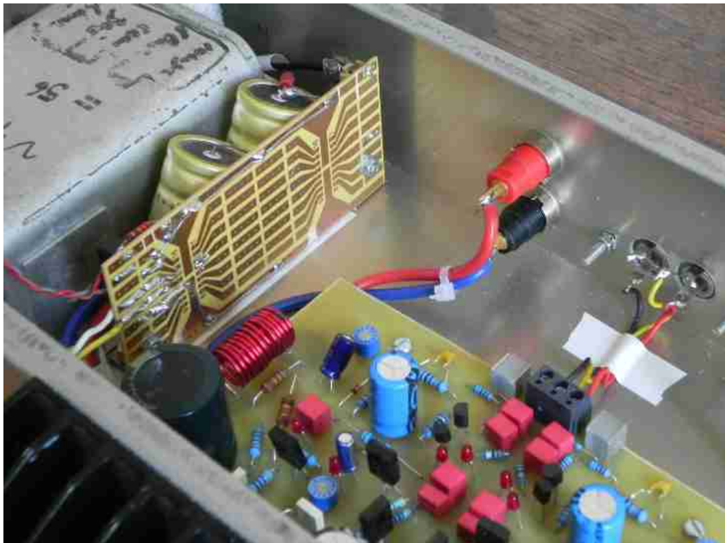
Fig006. The power supply is mounted on an original wafer Conrad. It hosts two SIC-SAFCO capacitors of 2200 uF, 63 V.
