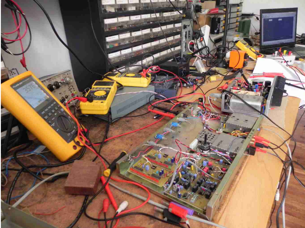
Fig051. The test bench. On the right, from the first plane, the generator-distortion meter, Renardson the amplifier. Basically, the computer displays spectrum analysis.
