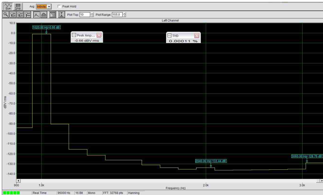
Fig061. The amplifier 3.6V vacuum: -133 dB H2, H3 -129 dB THD 0.00011%
