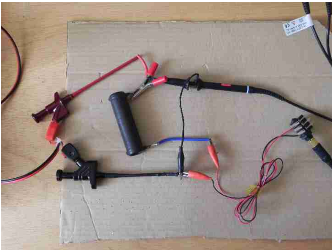
Fig023. Close-up view of the connection of the right channel to the headphone with series connection of a resistance of 8 ohms. The left and right channels of 6.35mm are connected together.
