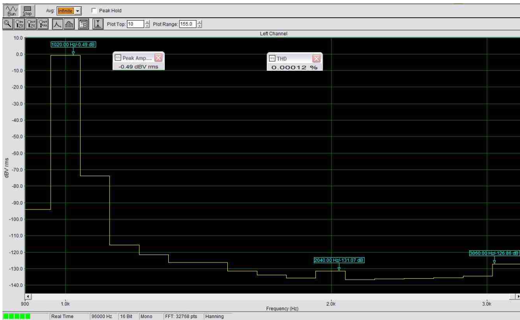
Fig065. Amplifier The 3.6V 16.8 uF: -131 dB H2, H3 -127 dB THD 0.00012%.
