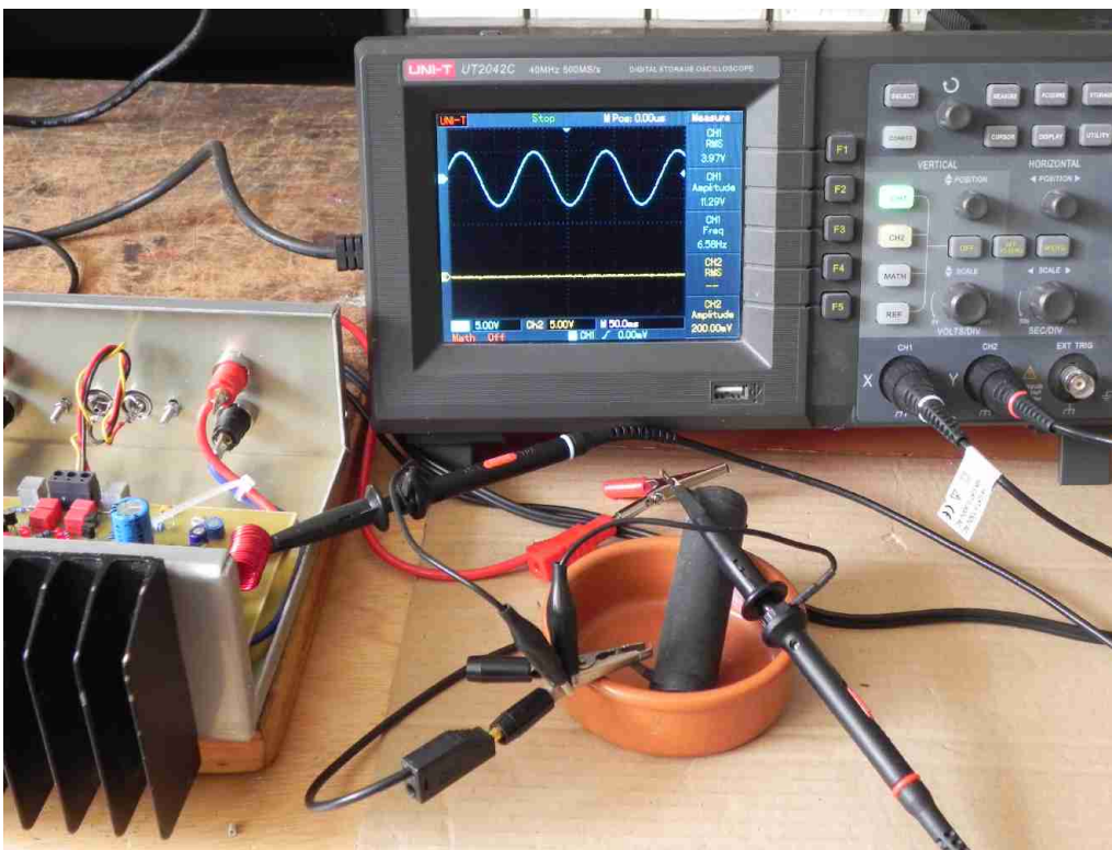
Fig035. Disconnecting the alligator clip of resistance. This is not very visible, it is placed back from the tip of the probe and merges around with it.
