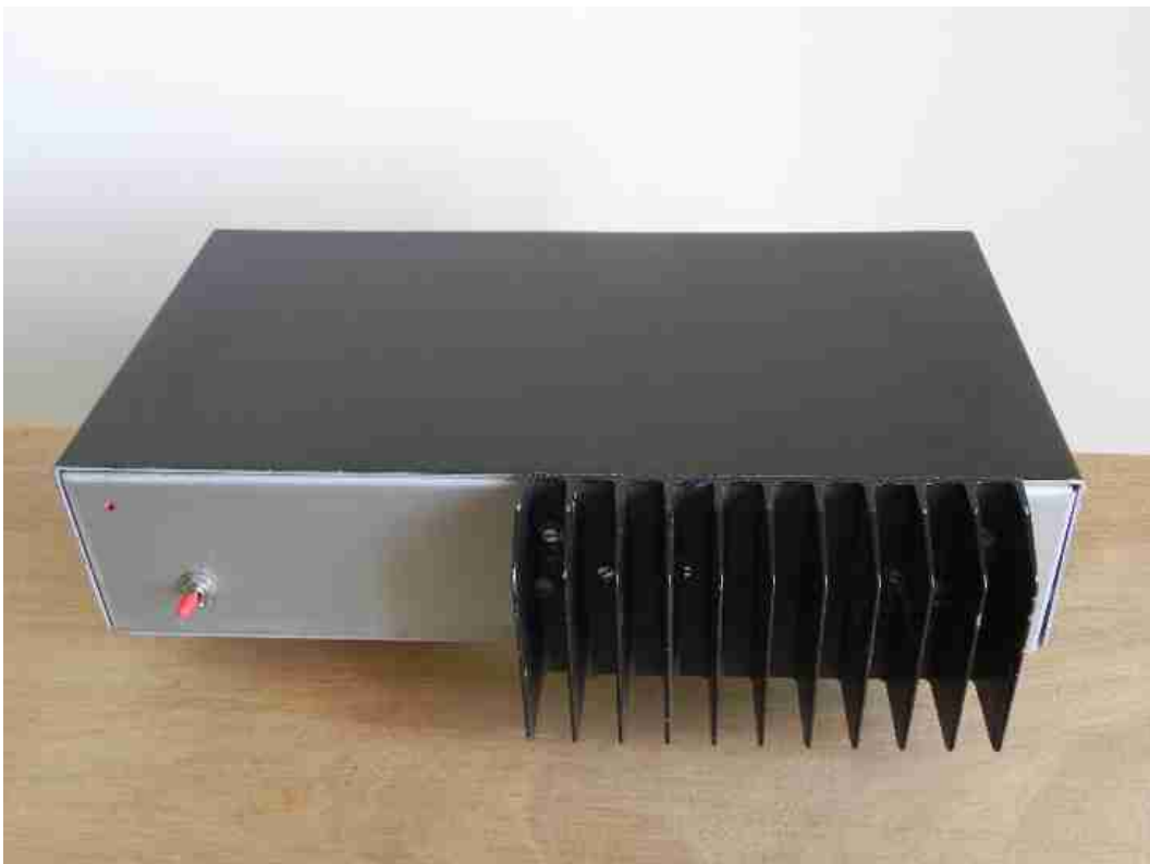
Fig002. Final assembly housing Teko 300 x 160 x 70mm. In use, it will be installed on a support, the radiator projecting from the lower face.
