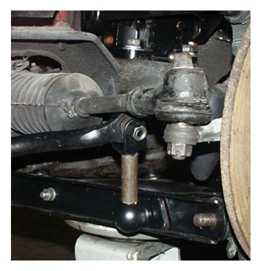
The sway bar eye is much closer to the tie rod, but still clears it by at least a quarter of an inch and the arm of the sway bar is much closer to level and thus pulls the link at much less of an angle as the suspension travels through it's normal range..
