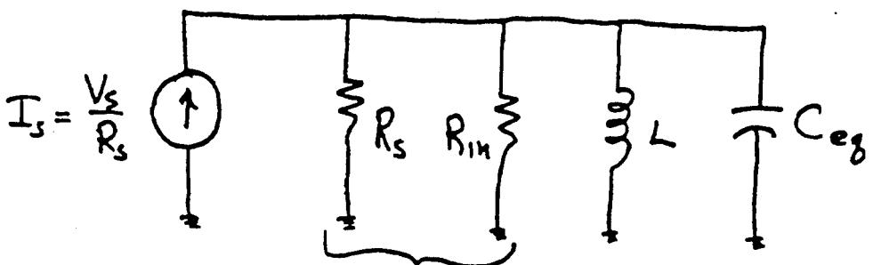
$$R_{eq} = R_s \parallel R_{in} = 250\Omega$$
