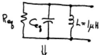
$$Q = f_0/B = (10 \text{ MHz})/(500 \text{ kHz}) = 20$$
