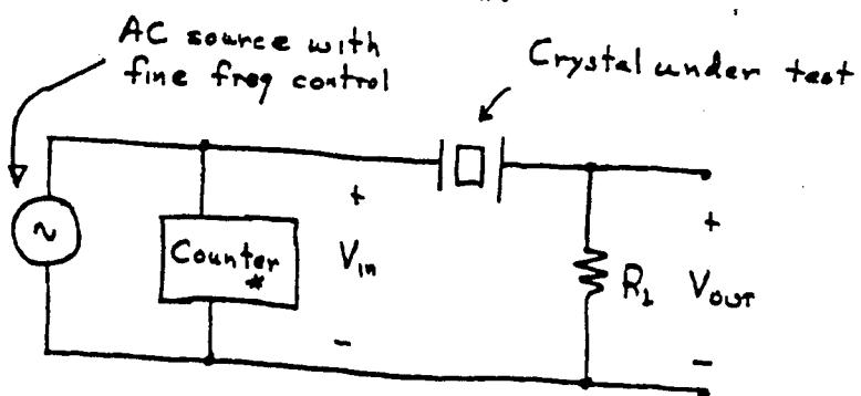
Use the counter to accurately measure the frequency of the source. Choose  $R_L \approx R_s$  of the crystal. Start with about  $50 \Omega$  and adjust as needed. Observe the voltage transfer function magnitude  $|V_o/V_{in}|$  which will appear much like the sketch shown on the next page. From the plot, determine the peak  $A_{max}$ ,  $f_s$  at which the transfer function peak occurs, the half-power bandwidth  $B$  of the peak, and  $f_p$  which is the frequency of the null.
