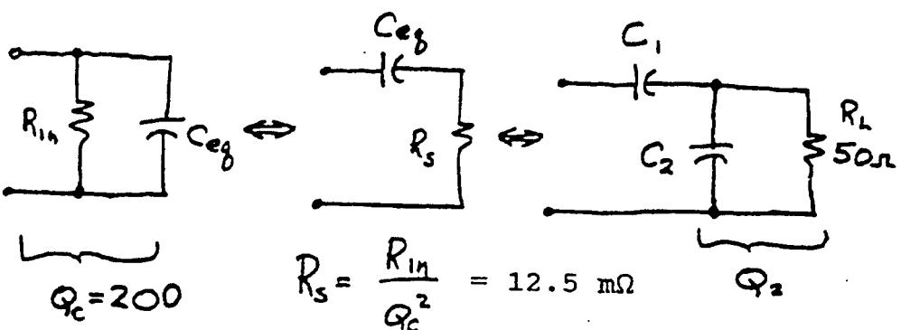
$$Q_c^2 = R_L/R_s = 63.24 = \omega_0 C_2 R_L \Rightarrow C_2 = 20.13 \text{ nF}$$
