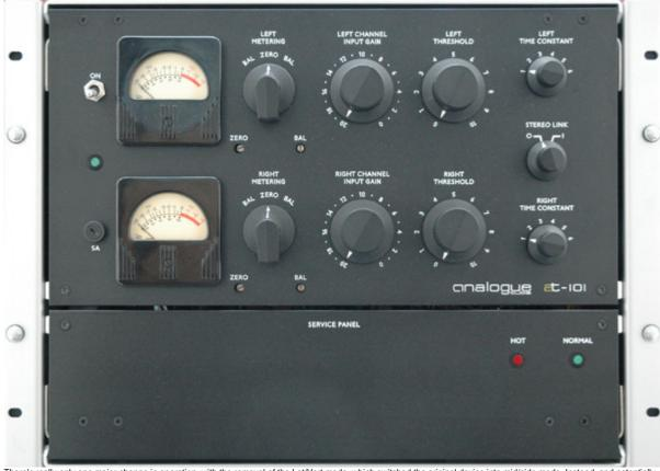
There's really only one major change in operation, with the removal of the Lat/Vert mode, which switched the original device into mid/side mode. Instead, and potentially more useful for the studio user (mid/side compression is normally associated with mastering, not tracking), the AT101 has a stereo link control, meaning both channels can be controlled by the knobs of channel one.
