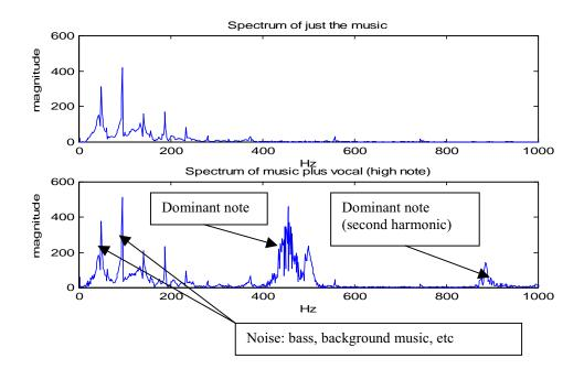
Thus, the pitch detection algorithm simply works as following: to search in the frequency domain from 100 to 800 Hz and find the frequency bin that has the maximum energy.
