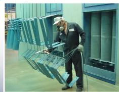
Our Powder Coating facility is 4'9" wide X 7'1" tall X 19' deep with an 8' center hook and operates in batches.
