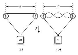
$v = \sqrt{\frac{T}{\mu}} = \sqrt{\frac{78.9 \text{ N}}{0.00100 \text{ kg/m}}} = 281 \text{ m/s}$
