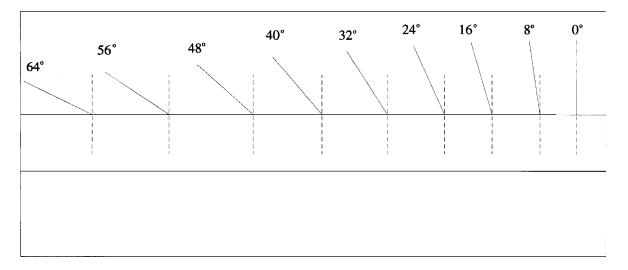
After completing the table below, make a graph plotting  $\sin i$  as the ordinate versus  $\sin r$  as the abscissa. Draw the straight line that best fits the plotted points. The slope of this line is the ratio of  $\sin i$  to  $\sin r$  and is therefore equal to  $n_g$ , the index of refraction of the glass block.
