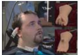
Control of a robotic hand using neuronal signals directly recorded from motor cortex. 2004 www.cybnetics.com
