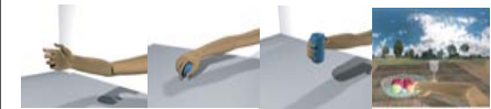
Virtual arm with multiple degrees of freedom. Using a combination of context sensitive controllers, a low bandwidth BCI signal can achieve simple tasks like reach-grab-fetch. (Johns Hopkins University)
