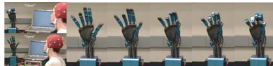
Two state motor imagery, combined with adaptive controllers, used to open and close a robotic hand. (Johns Hopkins University)
