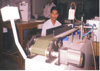
A new fiber optic sensor developed in the lab as a B. Tech Project, when attached to this system, enhanced its abilities to count number of accepted/rejected pieces, check dimensions, and belt jamming, etc
