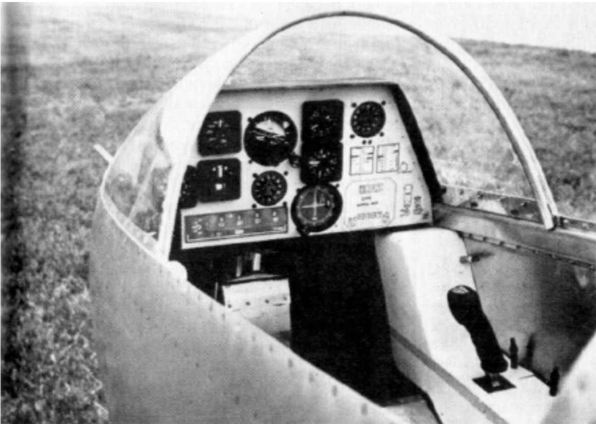
Trim cockpit of BD-5D jet features sidearm control grip like a fighter, miniaturized avionics for IFR flight.
