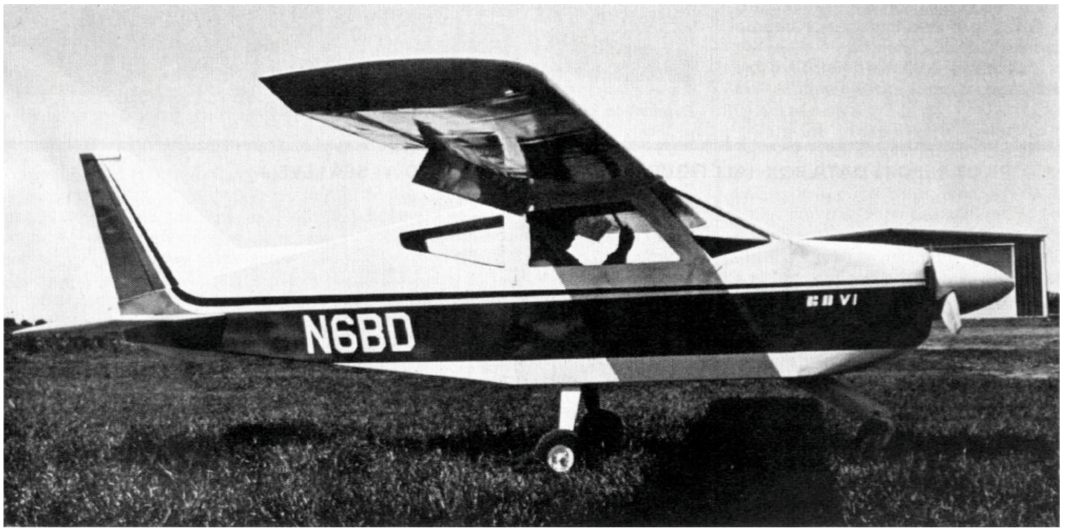
Newest homebuilt from Jim Bede is the BD-6, a single-place version of the popular four-place BD-4.
