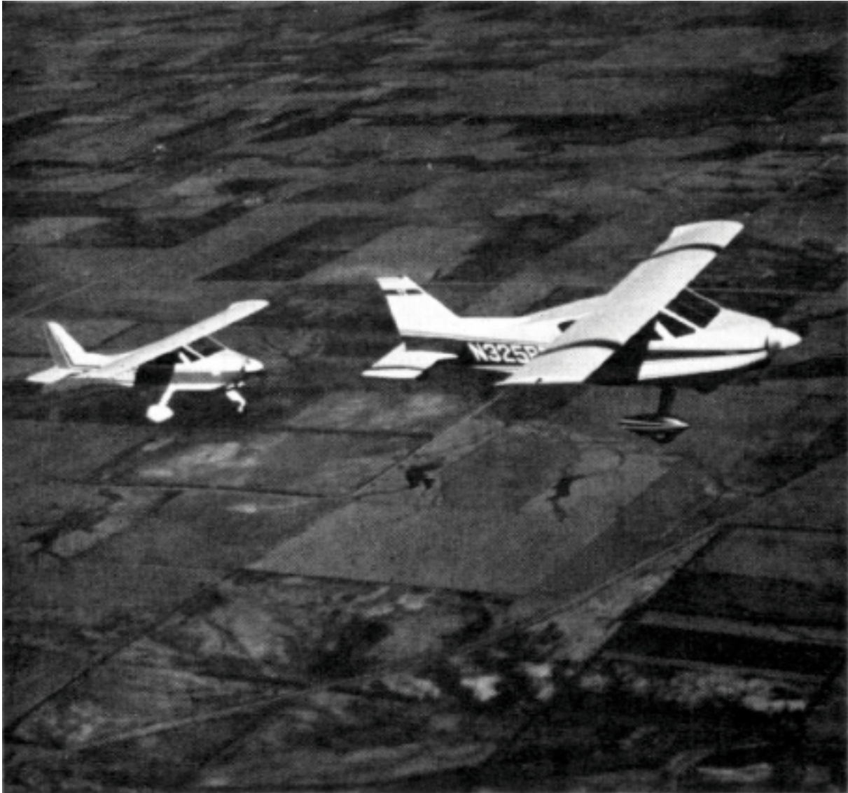
BD-6 is a spinoff of the high-wing BD-4, a four-place homebuilt that already is flying in quantity.
