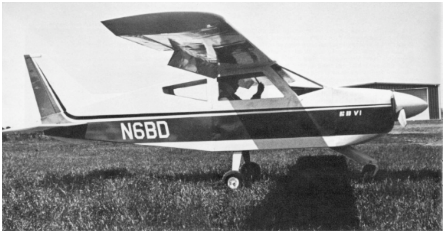
(Bede Aircraft Photo) The BD-6 with the flaps extended by means of the overhead actuating handle.
