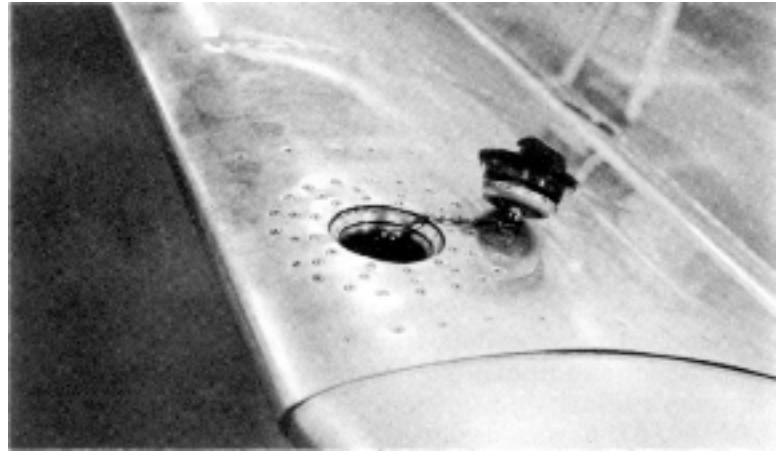
(Bede Aircraft Photo) "It starts up here and goes all the way down there!" That's the fuel filter hole for the BD-5J's wet wing. Along with a 15 gallon fuselage tank, total capacity is about 60 gallons.
