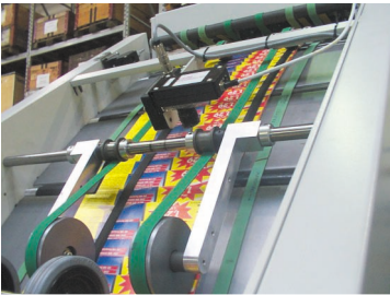
Optional fully-integrated digital image processing for extensive control tasks
