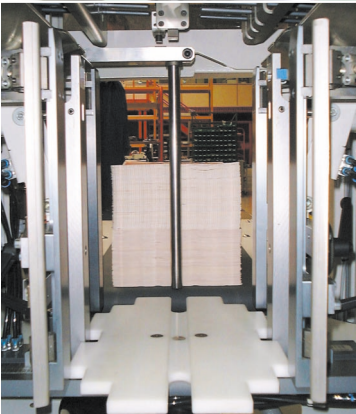
The electrically operated pusher and a telescopic belt for collecting the packets are responsible for making sure that the CS/1120 has the shortest possible cycle times.
