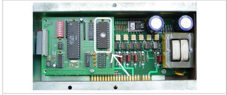
Begin by removing the fastener that holds the controller in place. Remove the controller and find the 28 pin EPROM located on the circuit board.
