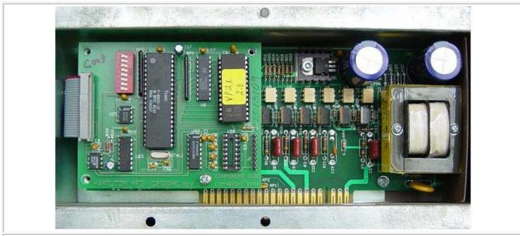
Finally, install the new EPROM into the controller, making sure that the notch on the EPROM is matched up with the notch on the board.
