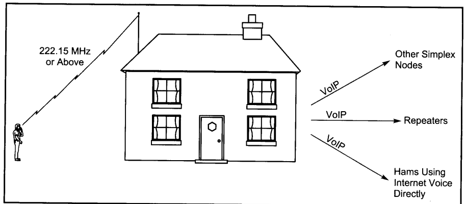
Figure 2—A diagram of a VoIP simplex node. If a control operator is not physically present at the station location and the node is functioning with wireless remote control, the control link must operate above 222.15 MHz. See the sidebar, “Is It Legal?”.
