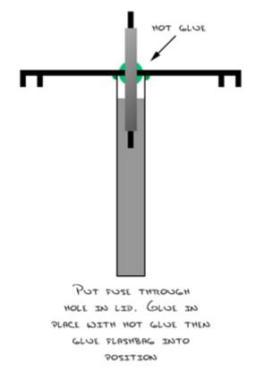
In the meantime, the canister was filled with one layer of stars on the bottom. Then a sort of "canulle" was prepared, a paper cylinder slightly wider and shorter than the flash bag consisting of two layers of paper, and held in the middle of the film canister while the stars were filled around it. Leaving a little space for the lid on top, not filling the canister with too many stars, the canister is now ready for the final assembly.
