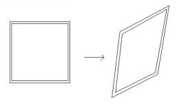
*I*n order to prevent the truss from changing shape (racking) or moving, the joints must be rigid. To rigid is to keep the members remain a certain angle with one another all the time
