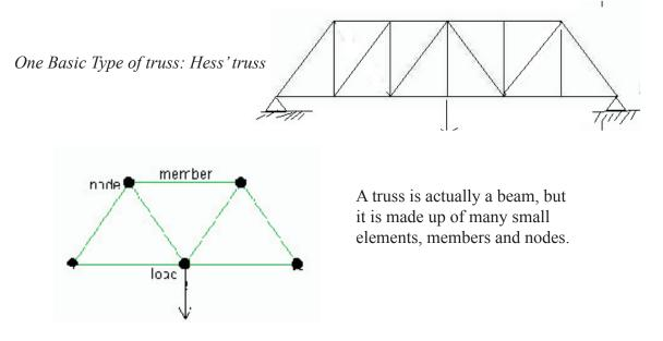
*Members* make up trusses. Truss is formed by straight members connected at their ends by hinged connections to form a stable configuration.
