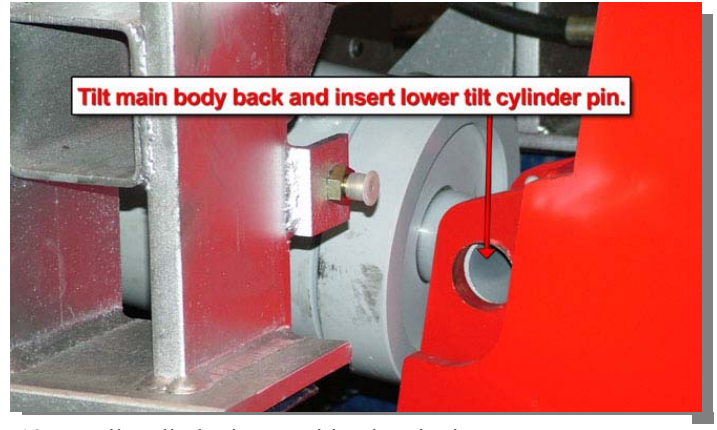
12. Put tilt cylinder into position by pinning.
