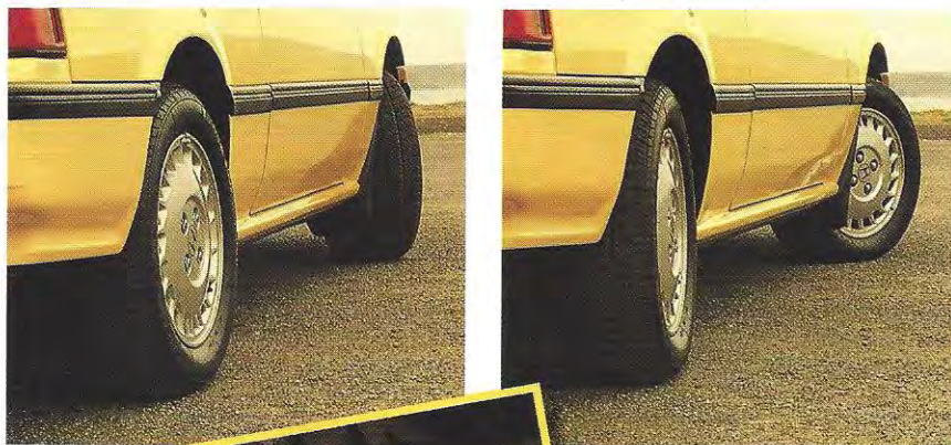
During normal driving, the rear wheels turn in phase to a maximum angle of 1.5 degrees, but for parking maneuvers, the rear wheels turn out of phase as much as 5.3 degrees.
